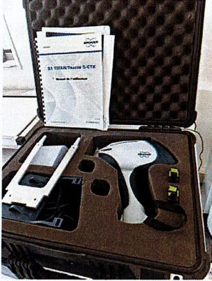
A Bruker Titan Tracer 5/CTX spectrometer is shown inside its brown, padded carrying case. The instrument is white and black, and the case is open, revealing the device and some manuals.                                                                                                                               |  |  |
