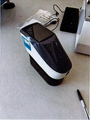
A white and black YS 3010 spectrophotometer is shown on a light-colored surface. It has a small display screen and a sample compartment. A black pen is visible next to it for scale.                                                                                                                                               |  |  |
